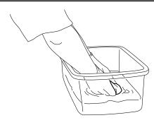
b. After cleaning, squeeze the air filter element to remove the excess solvent.
