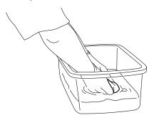
e. Thoroughly rinse the air filter element with water, and then let it dry.
